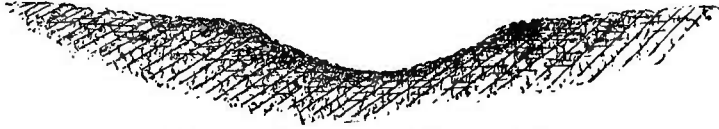
Fig. 13. Properly made open ditch.
